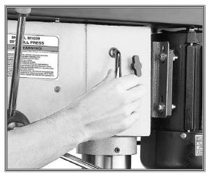
Figure 24. Using the belt tension lever.
